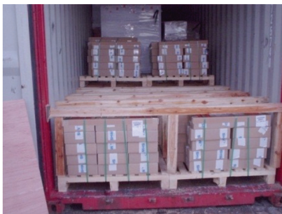
Figure 7.2 Timber temporary floor
