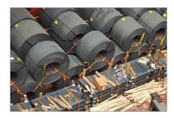
**STEEL COILS ON HOLD** Previous method Steel banding > converted to Cordlash 200.
