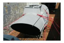
MACHINERY ON HOLD Previous method Steel Chains or Steel Wire > converted to Cordlash 750 or 1500.
