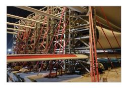
**BLADES ON DECK** Previous method Steel Chains > converted to Cordlash 1500.
