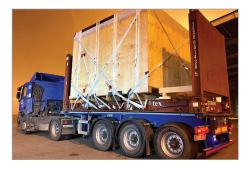
**CRATE ON FLAT RACK** Previous method Steel wire > converted to Cordlash 750.
