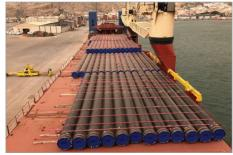
**FIBER & STEEL PIPES ON DECK** Previous method Steel Wire > converted to Cordlash 1500.
