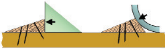
Figure 7.7 Properly cut and nailed wedges
