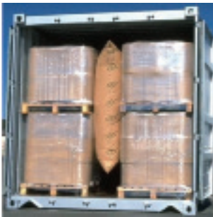
Figure 7.9 Gap filled with a central dunnage bag
