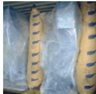
Figure 7.10 Irregular shaped packages blocked with dunnage bags
