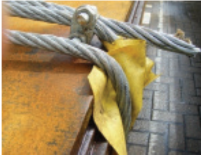
Figure 7.11 Poor edge protection
