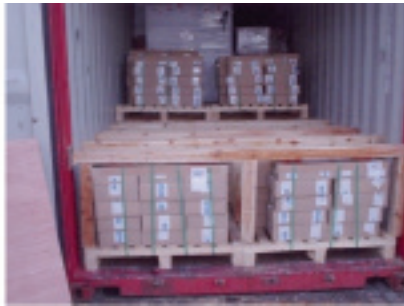
Figure 7.2 Timber temporary floor
