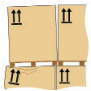
Figure 7.25 Without intermediate board
