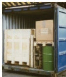
Figure 7.28 Mixed stow, use of pallets
