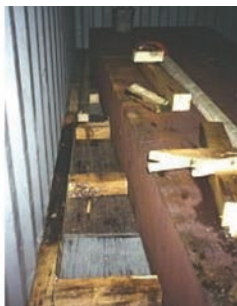
Figure 7.45 Transverse blocking of steel slab
