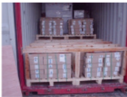
Figure 7.2 Timber temporary floor
