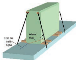
Figure 7.39 Direct lashing against tipping
