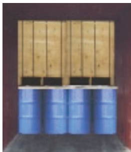
Figure 7.27 Mixed stow, dry over wet goods
