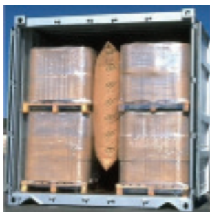
Figure 7.9 Gap filled with a central dunnage bag
