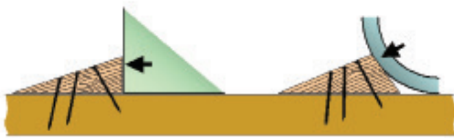
Figure 7.7 Properly cut and nailed wedges
