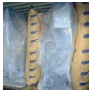
Figure 7.10 Irregular shaped packages blocked with dunnage bags
