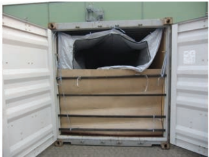
Figure 7.54 CTU with liner bag for accommodating a sensitive bulk cargo
